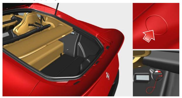
To release the lock and open the fuel filler flap manually, pull the cable on the right hand rear side of the engine compartment.
