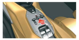
When "Automatic" mode is selected, the system automatically shifts UP and DOWN in relation to vehicle speed, engine speed and the torque/power requested by the driver.
