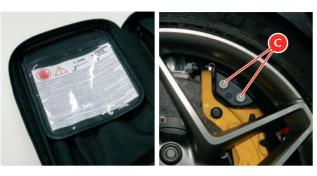
Once the electric parking brake has been released manually, at the next key-on, an error code is generated by the EPB node and the specific symbol and the relative message are displayed on the left hand TFT display: "Parking Brake system revision. Go to dealer".
