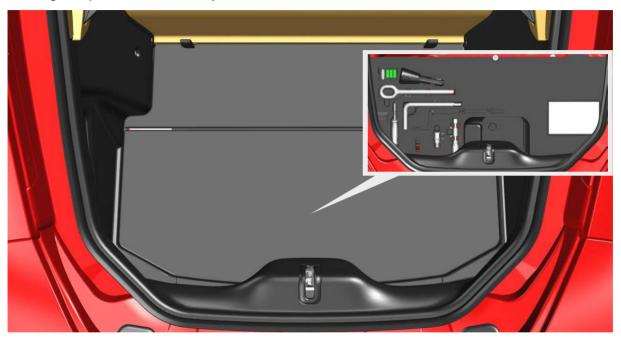
The tool bag, emergency tyre inflation and repair kit and spare wheel (if supplied) are kept in the luggage compartment.
