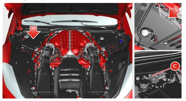
The battery is situated on the right hand side of the engine compartment. To cut off the power supply from the battery to the electrical system, use the quick release lever C situated on the left hand side of the battery to loosen the terminal clamp from the negative terminal of the battery.
