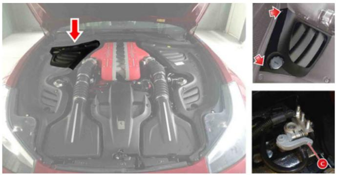
To cut off the power supply from the battery to the electrical system, use the quick release C on the left side of the battery. Use the locking lever to loosen the terminal.
