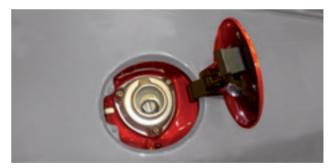
This vehicle has a capless filler neck for fuelling. This system allows you to refuel by opening the fuel filler flap and simply placing the nozzle in the filler neck without having to unscrew a cap and screw it up again. Two flaps placed in series, both with airtight seals, act as a cap. The external flap is locked by a series of "teeth" and the only way to open the external flap correctly is by inserting a petrol pump nozzle.
