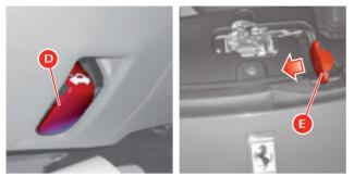
To unlock the engine compartment lid, pull the lever D underneath the steering column.
