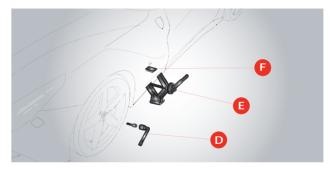
• Loosen the five wheel stud bolts approximately one turn each using wrench **D** supplied.
